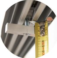
12. First Trolley Bracket Screw the first Trolley Bracket into the 'pocket-end' of the closer cassette until it measures 25mm from the underside of the head to the bottom of the Trolley Bracket.
