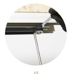
To tighten the belt, slide the screwdriver between the guide roller and buffer and lever tightening the belt. While the belt is tight tighten the grub screw to hold the tension.
