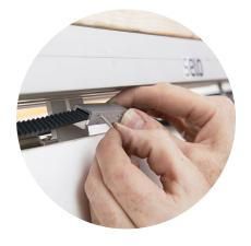
Unbolt the other carrier plate and insert the grooved pin into the belt.
