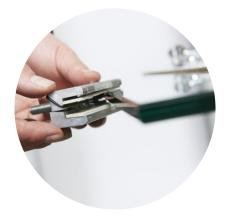
**5.**Place the clamps on the glass leaf and tighten the bolts.
