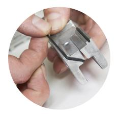
Put one rubber gasket into place looped round as shown.
