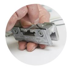
Cut 2 lengths of rubber gasket and fit into the top grooves of the other side of the clamp.
