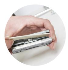
Place the clamp pads into place using the self-adhesive point holders. Make sure the correct pads are used for the thickness of glass being used.
