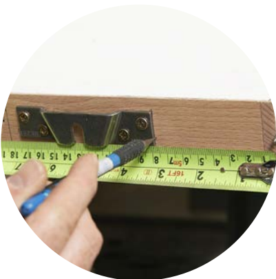
1. Fix the gear Brackets 80mm from edge of the Doors.
