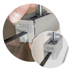
Select the right end cap to suit the glass thickness. Cut the section out to enable the cap to slide over the glass and clip onto the end of the clamp.
