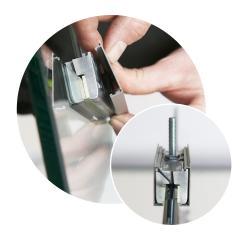
STEP 7 Fit the cover plates by hooking them on the top and pressing down until they click into the place against the glass.
